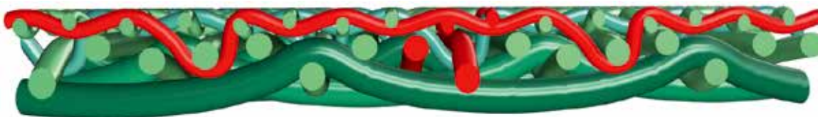
Primoselect concept with only a single binder yarn: Lower void volume, reduced caliper, faster dewatering
