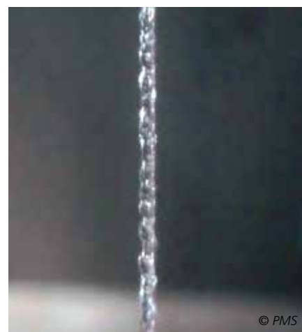
A turbulent jet is evidence of defective nozzles
