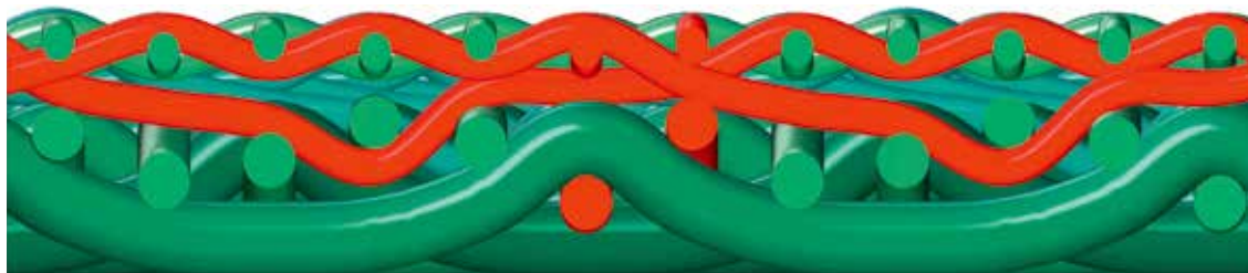
Standard SSB with paired binder yarns and higher void volume
