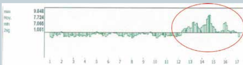
Moisture profile before the reel / higher moisture on the drive side
