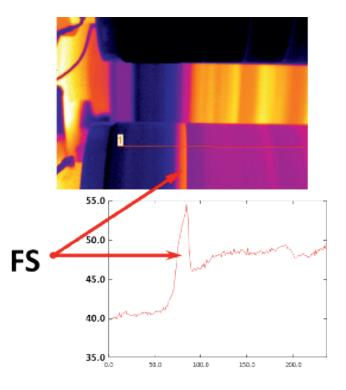
As a rule, starting at the reel spool, images are taken, tracking the error in the machine. In the area of the forming section no temperature difference between high and low dryer contents is detectable most of the time, as fibres and water still have the same temperatures at that point.
