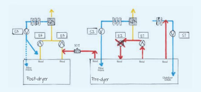
This effect was intensified by the design of the exhaust duct, which impeded air extraction. Therefore, the heat exchanger did no longer work efficiently, and the hot air intake became noticeably colder. As a result, the paper sheet dried more slowly, and the customer was forced to reduce the machine speed considerably. And this with increased energy use! Matters were made worse by two very large holes in the air intake duct of the post-dryer,
