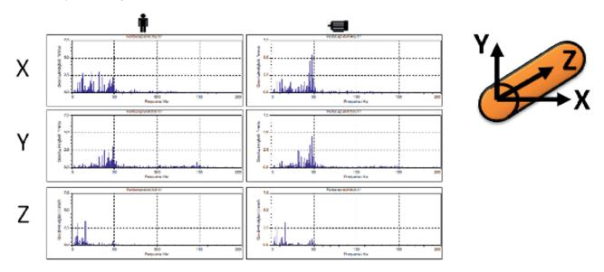
Thus, a graphic representation of the FFT is possible (see diagram). The acceleration sensors in the press section are primarily attached to the bearing housings of the rolls. Every measurement takes place simultaneously at the front side and the drive side of the respective roll.
