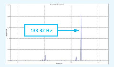
The technical specifications of the vertical screen showed that the rotor had four blades. This meant: Rotating frequency  $(33.33 \text{ Hz}) \times 4 \text{ blades} = 133.32 \text{ Hz}!$
