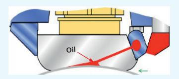
The shoe in this press was interrupted in the running direction of the machine. At this point pressure was created with oil (red in the diagram); this means the lubricant for the inside of the press belt is introduced directly into the shoe during operation. However, the oil could not be introduced in shut mode, which also concerned the nip profile measurement, because the press belt would have been saturated with oil.
