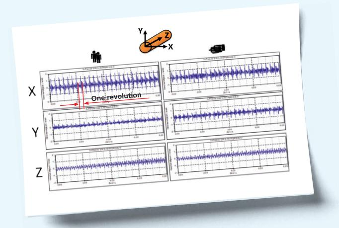
The time signal of the press belt in the shoe press showed clearly that once per rotation the belt swung/shifted horizontally. This led to extremely strong vibrations in the entire press section. The next day the belt was removed and checked. It was damaged on the inside over an approximately 30cm long area, which made the press section to vibrate once per rotation.
