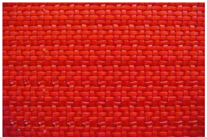
Fig. 3: Roll side – extremely dense, so that dirt cannot penetrate.
