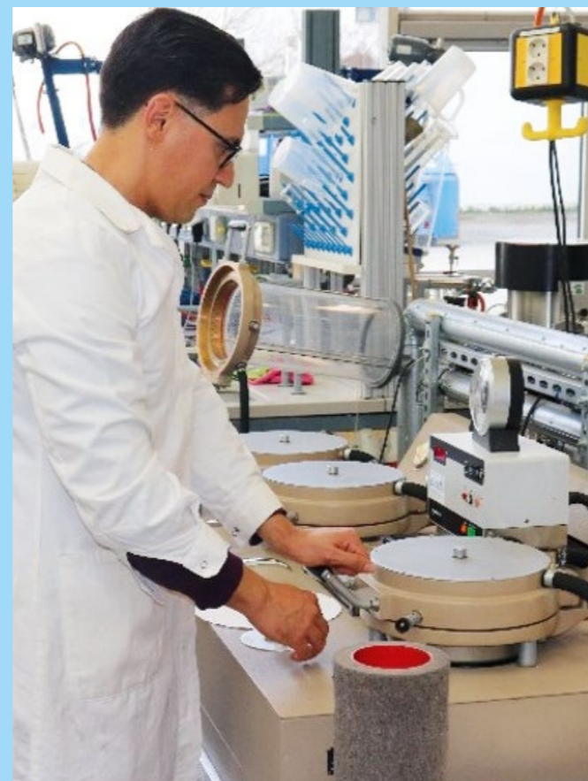
Laboratory sheet formation in the papermaking pilot plant
