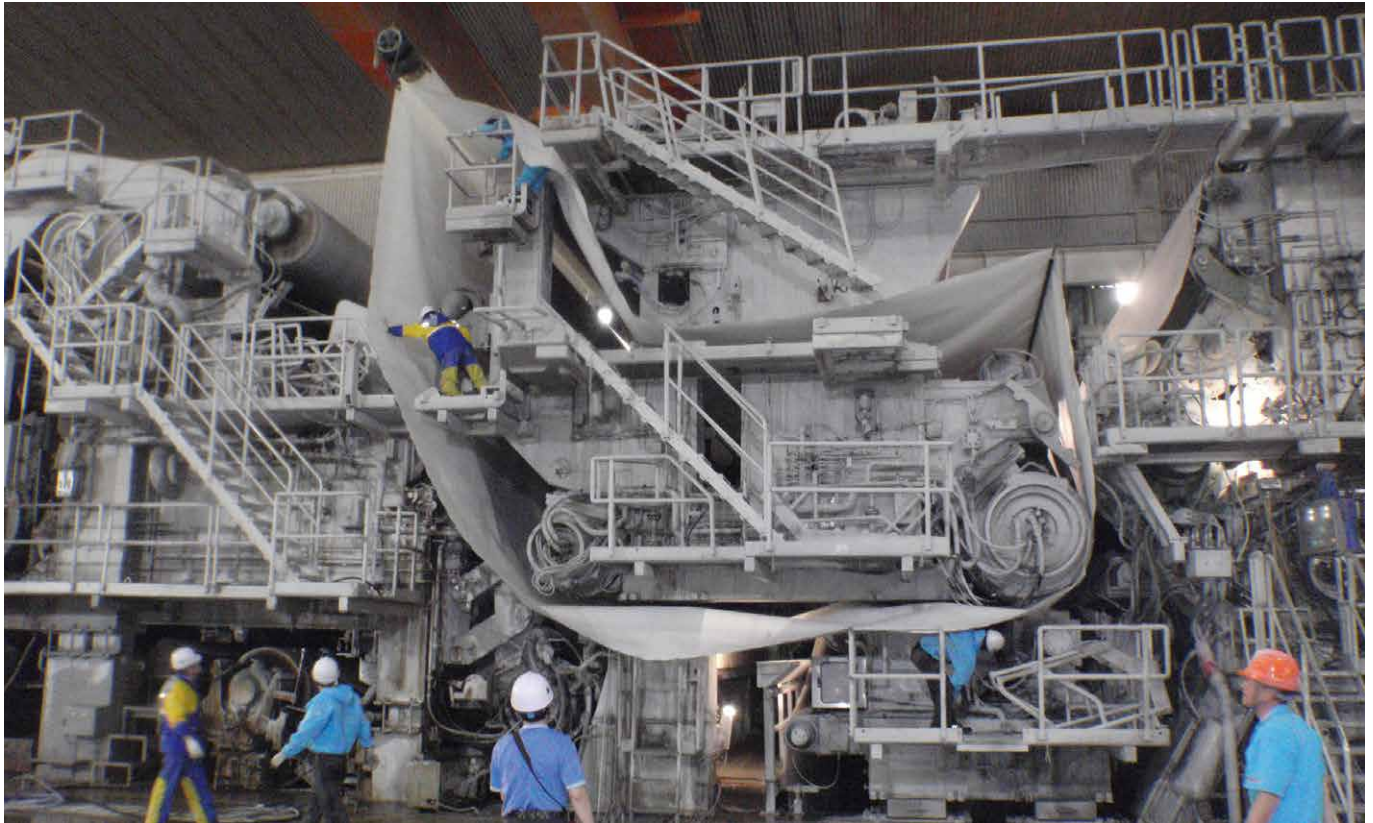
Pick-up felt installation on PM7
