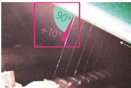
Fig. 9: Ideal angle of the water jets
