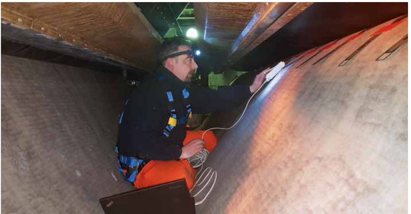
Nip profile measurements provide clarity
