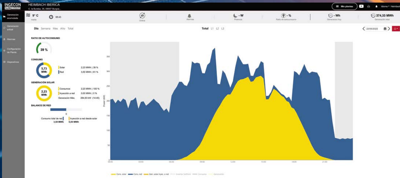
Under optimal conditions, the solar system covers up to 40 per cent of the daily energy requirement
