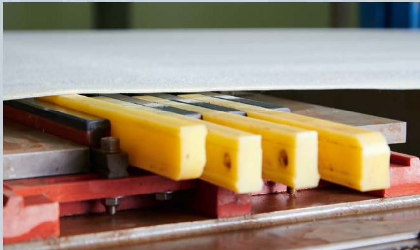
Fig. 11: Raised edge deckles on the Uhle box
