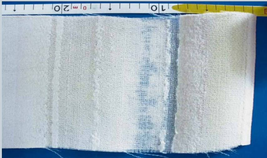
Fig. 10: Total loss of batt in the felt edge area
