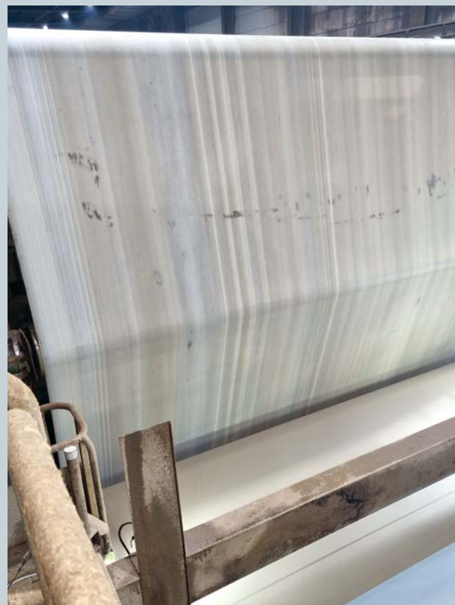
Fig. 6: Result: wet streaks in the felt
