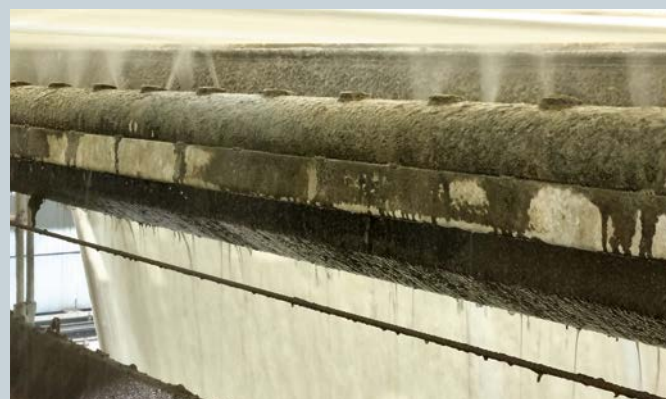
Fig. 5: Uneven water application
