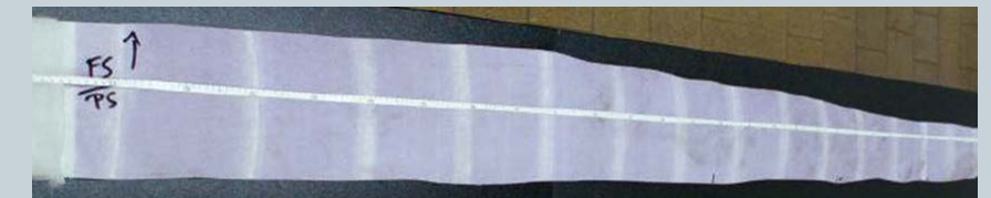
Fig. 8: Zonal felt wear visually identifiable in the used felt
