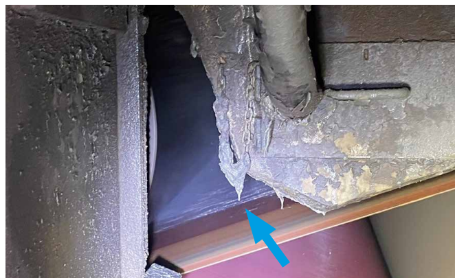
Fig. 2: Typical OEM save-all in easy position. Fast machine with high nip-dewatering, but a large part of the water is not captured. This leads to crushing, especially with old felts.
