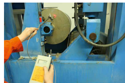
Fig.6: IR measuring probe to determine rotation frequency
