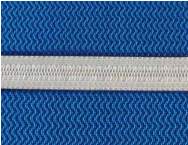
Spiral closing seam in a transport belt for the food industry
