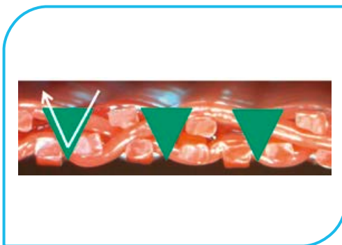
Fig. 7 The vertical funnel structure makes easy cleaning deep into the fabric possible and its small channels prevent dirt being pressed through the fabric onto the roll.
