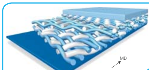
III.3 ATROMAXX.XF: Upper base layer with MD flat yarns
