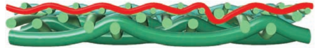
Figure 7. Primoselect on SC machine after a normal run – binder yarn is not abraded
