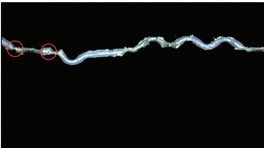
Figure 6. SSB with serious internal abrasion
