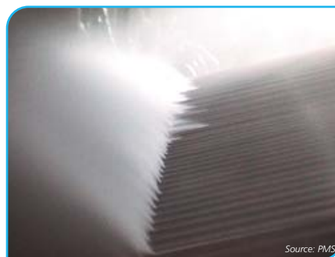
Fig.12 Water mist in the space inside the fabric return loop
