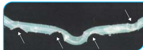
Fig.22 Machine direction yarn showing internal abrasion
