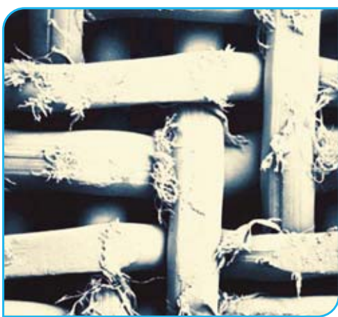
Fig.10 Fabric damage through excessive jet impact
