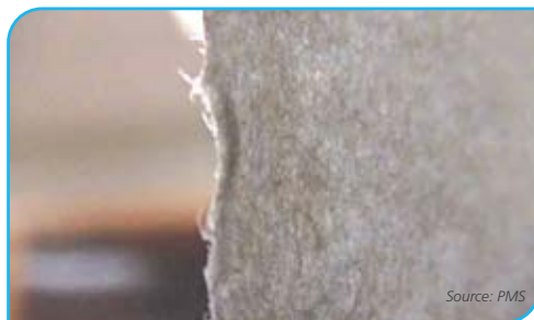
Ill. 1 Faults in the sheet edge
