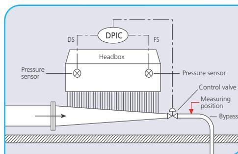
III.27 Schematic Layout of Pressure Sensors and Headbox Bypass
