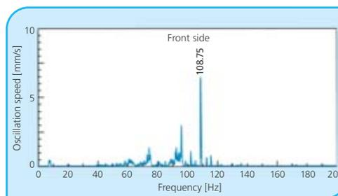
III.9 Total 4. Press oscillations, measured on top roll in nip direction
