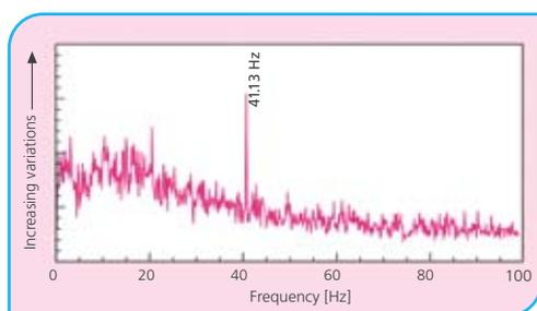
III.17 Variations measured in the forming section at 855.7 m/min wire speed
