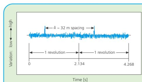
Ill.20 Trigger Signal Bottom Wire (Forming Section)
