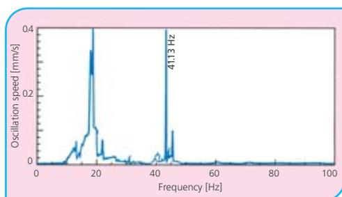
III.18 Oscillations of intermediate pressure screen in radial direction top; wire speed 855.7 m/min
