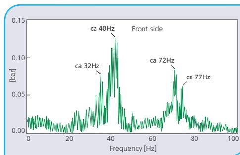
III.29 FFT pressure signal at headbox before change of control valve
