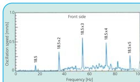
III.14 Total oscillations of stock mixing pump in axial direction
