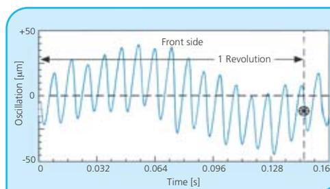
III.10 Synchronised time signal of the venter roll, measured on top roll in nip direction
