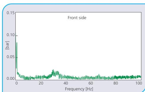
Ill.30 FFT pressure signal at headbox after change of control valve
