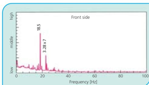
III.12 Variations in the sheet after the calender Forming wire shake frequency 3.28Hz, Stroke 7
