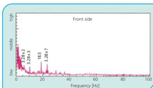
III.13 Variations in the sheet after the twin wire former Shake frequency 3.28Hz, Stroke 7
