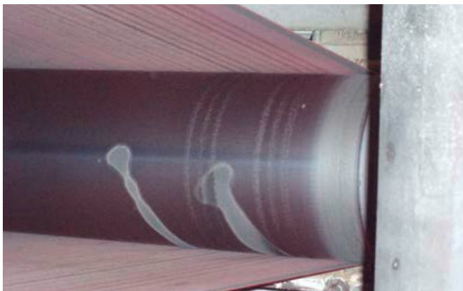
Deposits on the rolls are the result of contaminated dryer fabrics.
