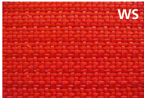
A smaller number of contact points as well as a reduced contact area on the paper side prevent adhesion of dirt and make cleaning more efficient. Conversely, the density of yarns on the roll side increases wear resistance.
