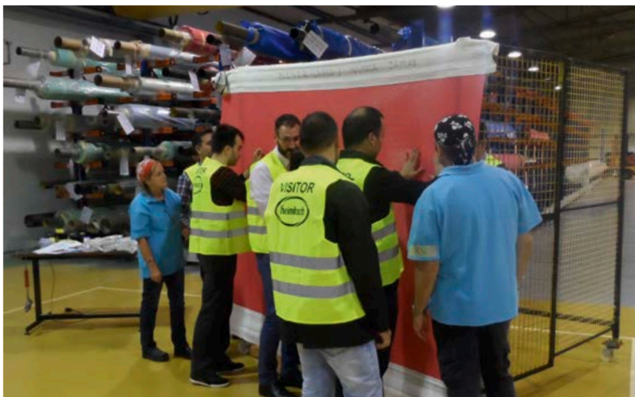
The working group repairing a damaged dryer fabric.
