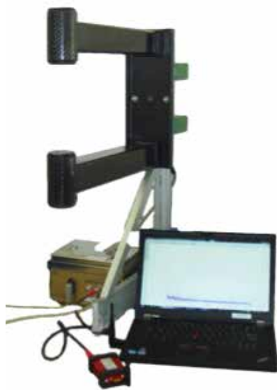
The “Odin” portable measuring fork is able to detect the root cause of vibrations.
