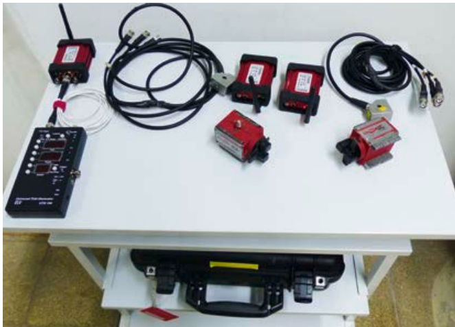
Fig. 1: The Heimbach TASK test kit at a glance: Below left is the "clock generator", which is used for offline synchronization. Top left and in the middle of the table are the three transmitters of the telemetry system, with which the specific values are determined (transmission range: approximately 150 m). Also shown is the "triaxial acceleration recorder" including two "contour magnets" used to inspect the x, y and z direction of the roll.
