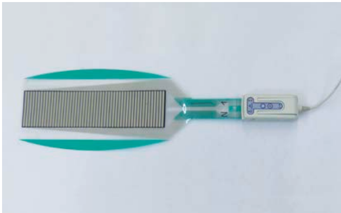
Photo 1: Measuring membrane and "multiplexer" in close-up.
