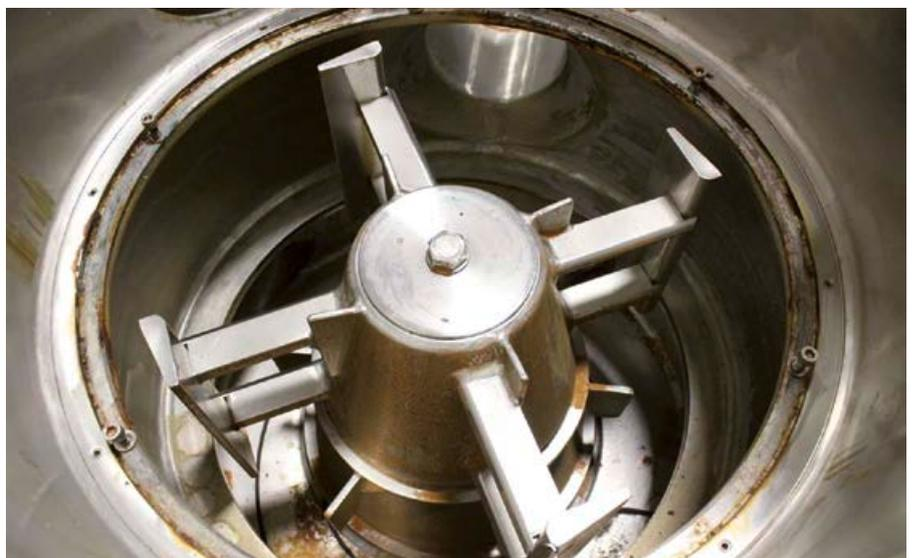
Photo 2: Vertical screen with four-blade rotor.
