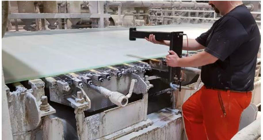
Photo 1: Measuring point 5 before couch roll.
