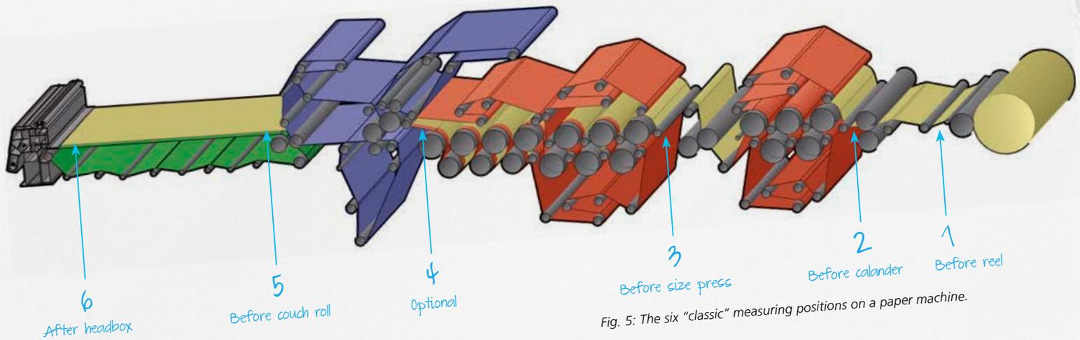
Fig. 5: The six "classic" measuring positions on a paper machine.
